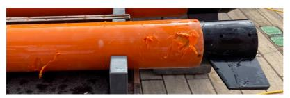
working hard in the field! The protective rubber coating of the magnetometer shows deep gouges, probably from a shark attack.
