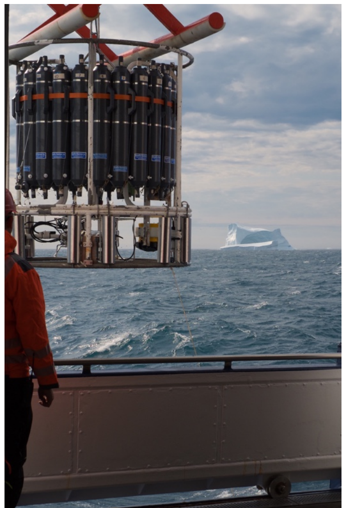
Recovery of the rosette water sampler with CTD close to the east coast of Greenland.
