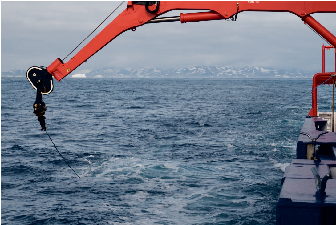
Tow fish hung from a crane on Maria S. Merian to collect samples of surface water for measurements of trace elements and nutrients.
