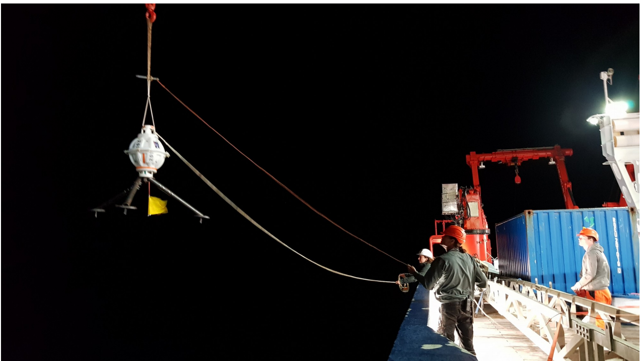
Recovered floatation bodies wait for being serviced. The last PIES is going to be deployed.
