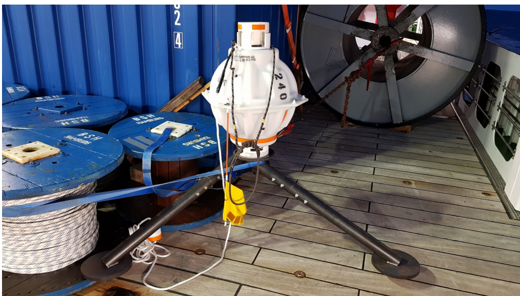
An inverted echo-sounder equipped with a pressure sensor (PIES) is waiting for its mission at depth.
