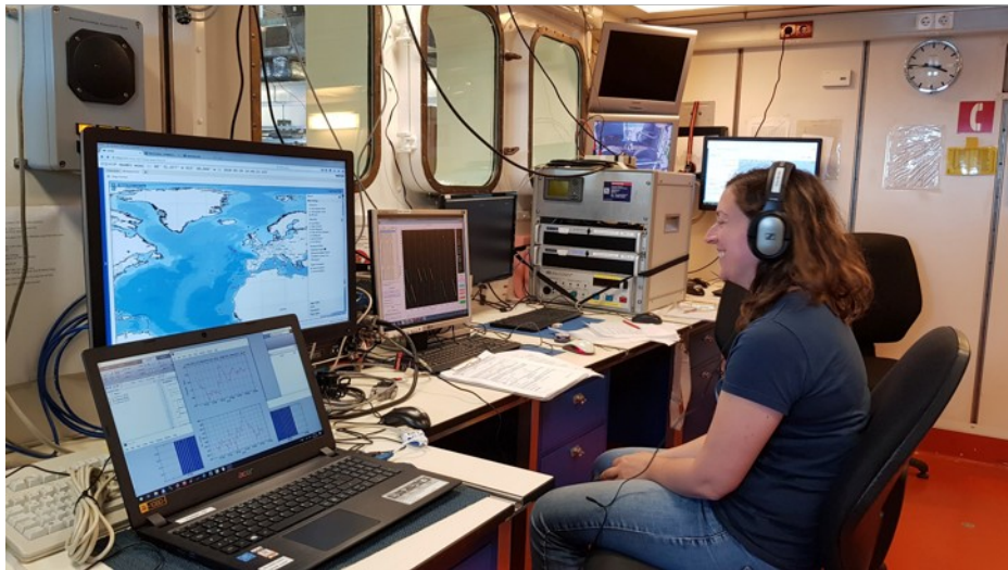
Top: Spooling the ropes onto wooden drums while recovering mooring EB-3. Bottom: Acoustic live transmission of the data recorded by PIES BP-32 (Photos: D. Kieke)
