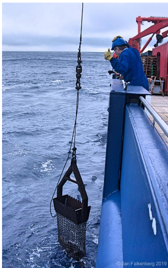
A successful chain dredge haul is on its way onboard (Photo: Jan Falkenberg)
