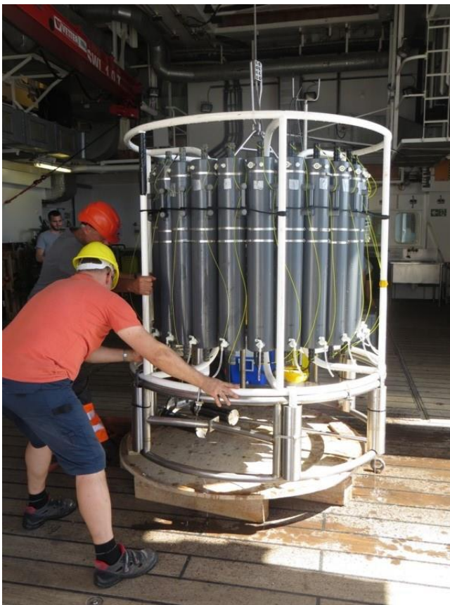
Fig. 1: CTD/Rosette returns to the hangar after deployment (Foto: H. Auel)
