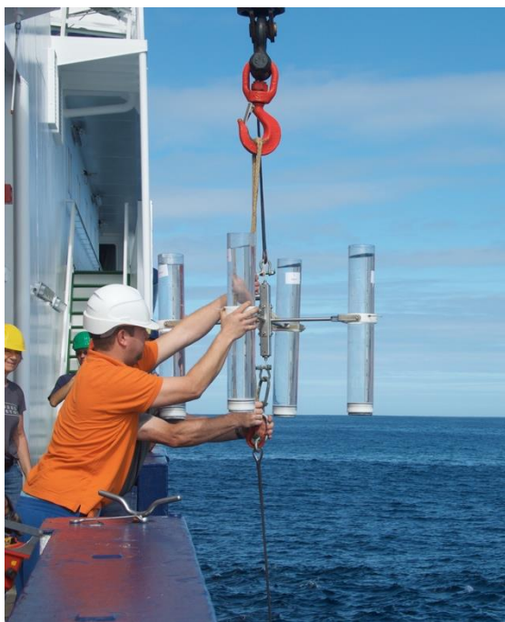
Figure 1: Left, recovering a drifting trap in the morning of 21.11.2018. Right, the harvest of the trap that collected particles at 100m water depth.
