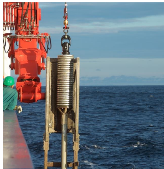
Figure 2. Left, Parasound Profile of the ocean floor in the research area, Right, The recovery of the gravity core GeoB 23303-2.
