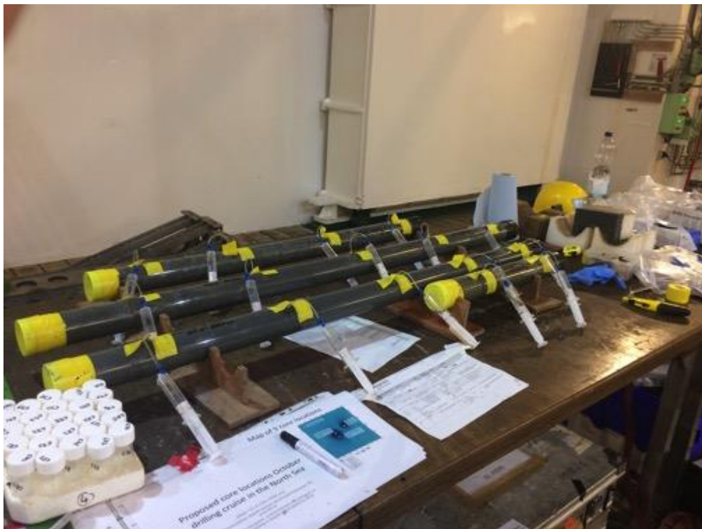
Figure 2: Pore water sampling of sediment core segments
