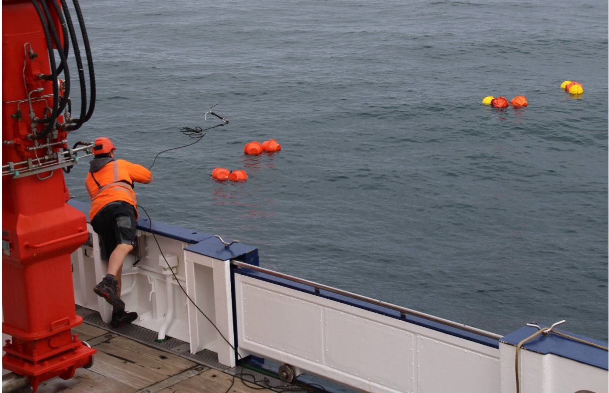
Fig. 2: A grapple is used for the recovery of a mooring. Photo: Dragonfly Ame Leathrum-Simons
