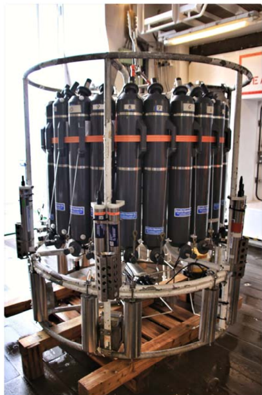
The water sampler is rigged with mooring devices (MicroCATs). These instruments were previously equipped with batteries and programmed accordingly.
