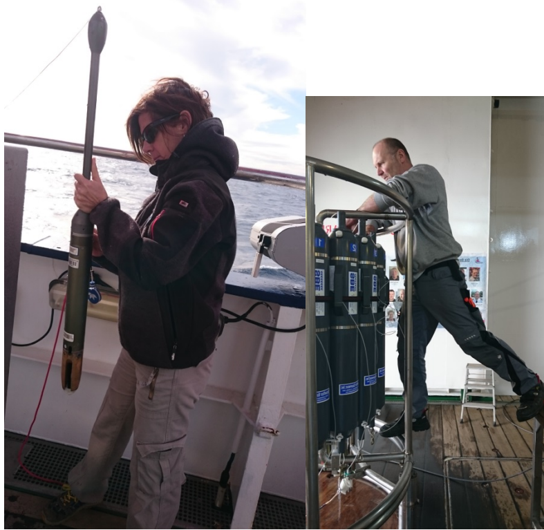
Fig. 2: Vanessa finished an uCTD-cast and Andreas is busy on repairing the CTD.
