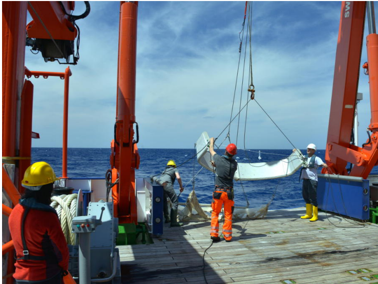
Figure 2: Deployment of the 0.5 mm mesh size Isaaks-Kidd Midwater Trawl (IKMT)
