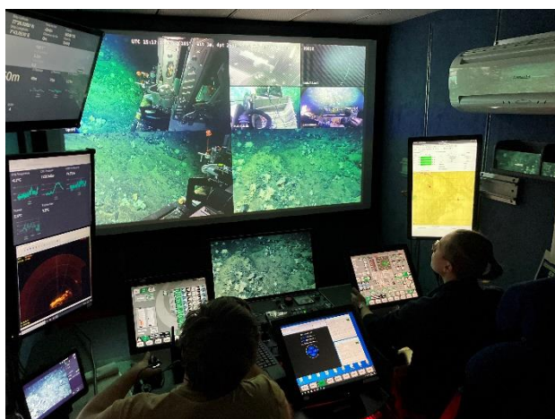
Figure 1: View into the pilot control room of MARUM ROV QUEST4000. From this fully equipped control container, the two pilots have control of all video cameras and steer the vehicle on the seabed (© Gerhard Bohrmann).
