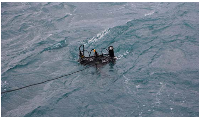
Deployment of the Satlantic radiometric profiler within Vaigat on the west coast of Greenland (Photo: Oliver Zielinski, ICBM, University Oldenburg)
