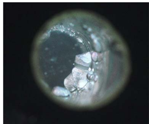
Figure 2: As the gas bubbles accumulate in a funnel, we could observe gas hydrates forming immediately at water depths within the gas hydrate stability zone. Copyright: MARUM University of Bremen
