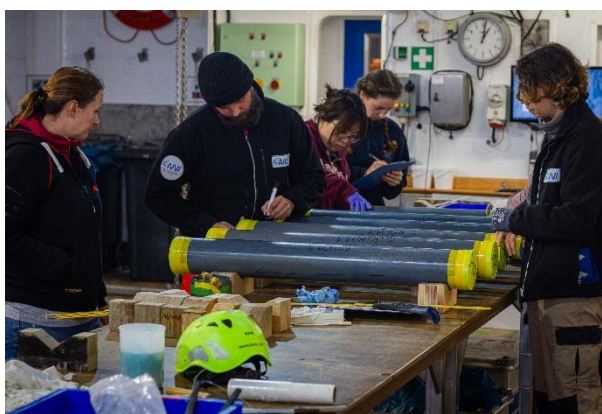
Figure 3: A sediment core in 1-m segments is brought into the hangar of RV MARIA S. MERIAN for labeling and sampling. Photo: S. ten Hietbrink.
