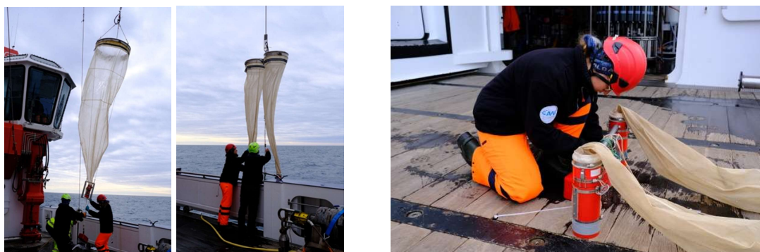
Photos Julia Oelker: Deployment of the large zooplankton net and the Bongo net; right: Isadora Jalil preparing the Bongo net.
