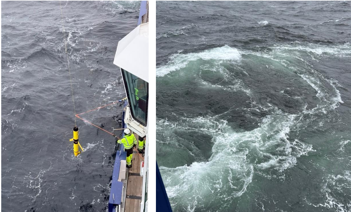
Figure 2: (Left) Glider recovery after a 13-day mission through an anticyclonic eddy west of the Greenland coast (Photo: Fehmi Dilmahamod). (Right) The greenish colour of the water, likely associated with the intense Labrador Sea spring bloom, with surface chlorophyll-a concentrations reaching up to 15 \text{ mg m}^{-3} (Photo: Eleanor Frajka-Williams)
