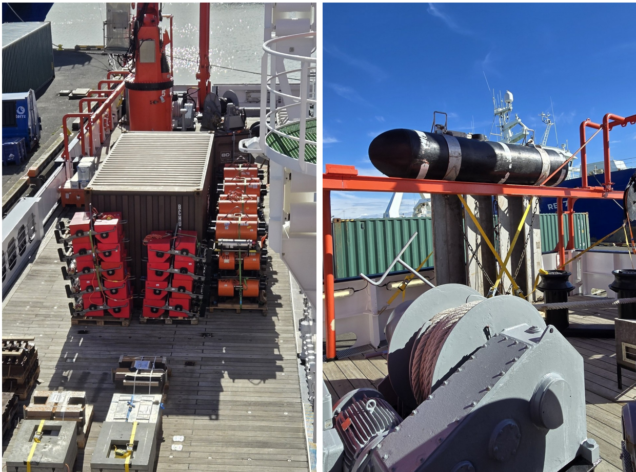
Figure 1: OBS, OBEM and their anchor weights (left) and the rigged trawl door of the P-cable system (right) on the deck of RV Maria S. Merian in the port of Reykjavik. Photos: I. Klaucke.
