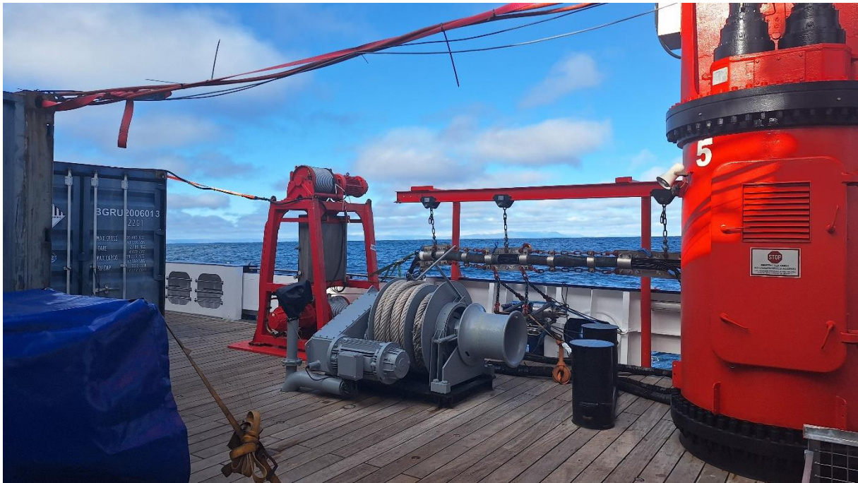
Airgun winch on the starboard side of RV Maria S. Merian.
