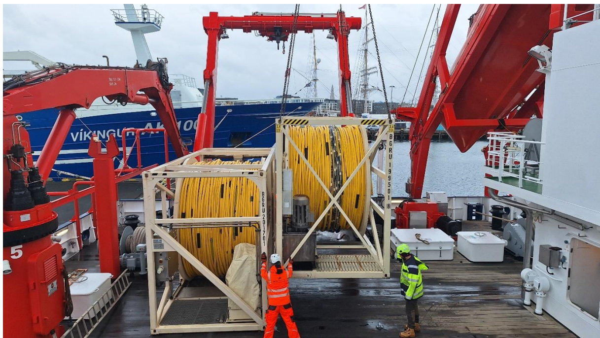
Loading of both seismic winches with more than 6 km of hydrophone cable.
