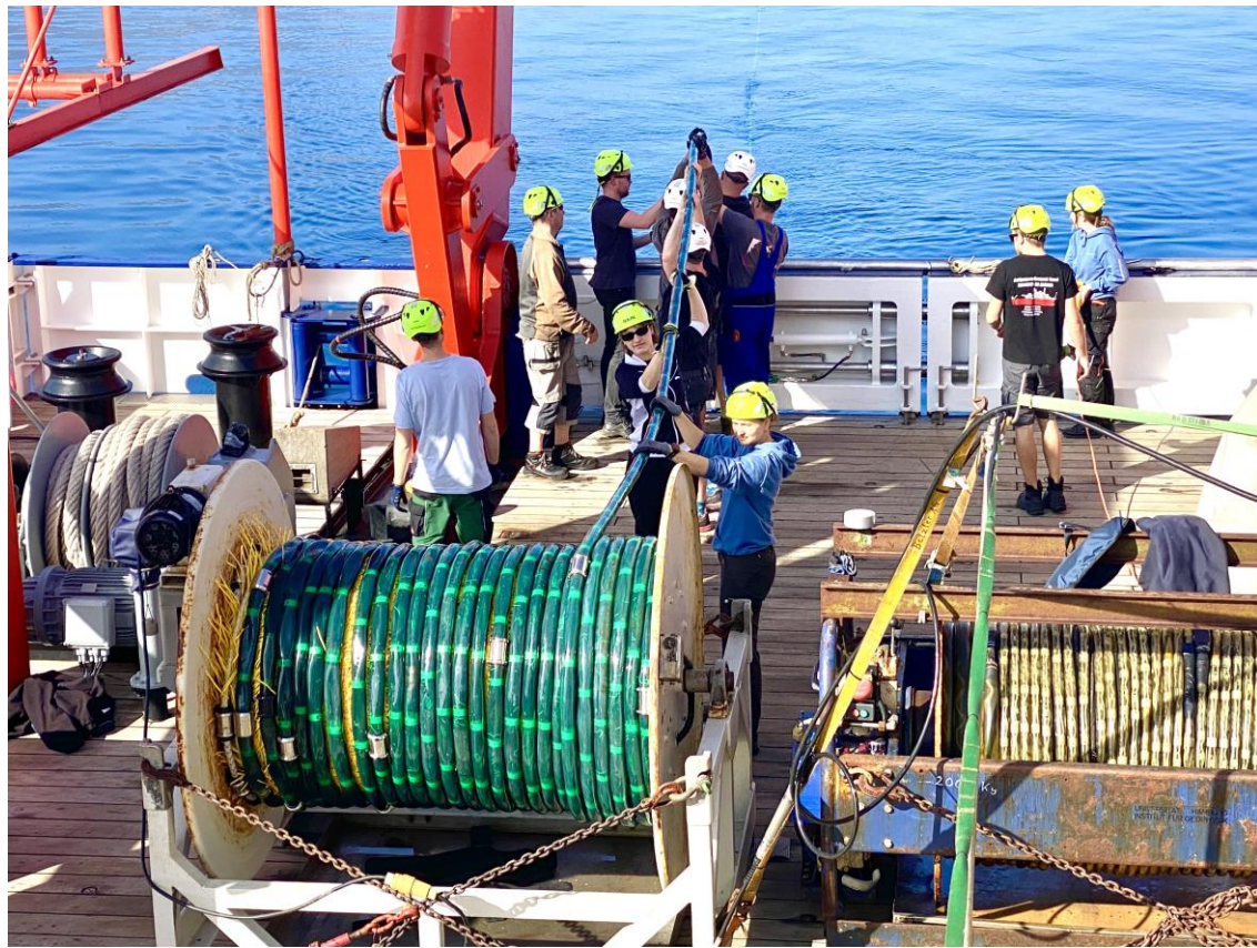
Figure 2. Deployment of hydrophone cable. Foto: H. Jähmlich.
