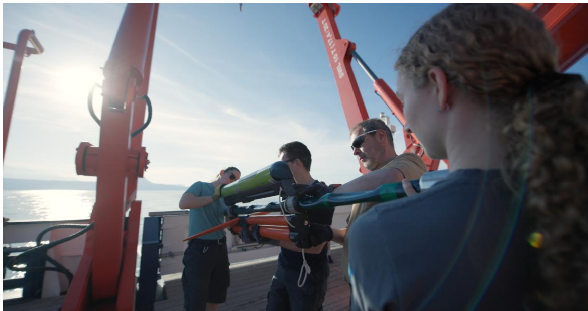
Figure 2: Deployment of the 800 m long receiver cable for the reflection seismic measurements. Foto: J. Vollert.
