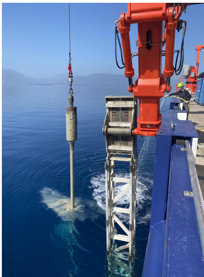
Figure 1: The Gravity Corer back from the seafloor. Picture: H. Jähmlich.
