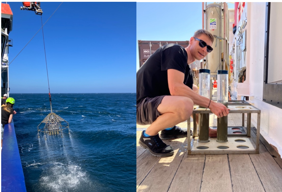
Picture 2. Recovery of the multicorer, collection of sediment (photo's: K. Zonneveld).
