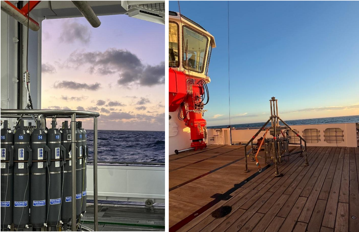
The CTD-Rosette (left) and the Multi-Sediment Corer (MUC, right) deployed during the MSM133 research expedition. The CTD-Rosette was used to collect water samples and measure conductivity, temperature, and depth, providing crucial data on the physical and chemical properties of the water column. The MUC allowed for the recovery of undisturbed sediment cores from the seafloor, enabling detailed analyses of organic matter composition and microbial activity in surface sediments. Both instruments were essential for investigating the vertical and lateral transport of organic matter in the Mauritanian shelf and slope regions. (Images provided by Julia Pamphile dos Santos).
