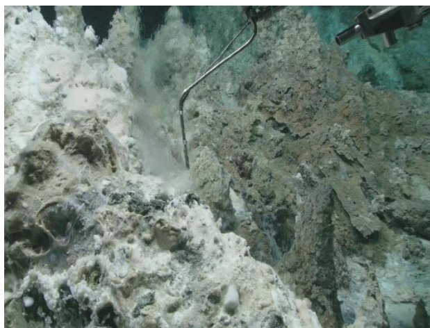
Figure 3: Sampling with a gas-tight IGT sampler at a fluid vent (shimmering spot) at the Nidhogg hydrothermal mound. The surrounding hydrothermal rocks are intensively covered with white microbial mats (© MARUM).
