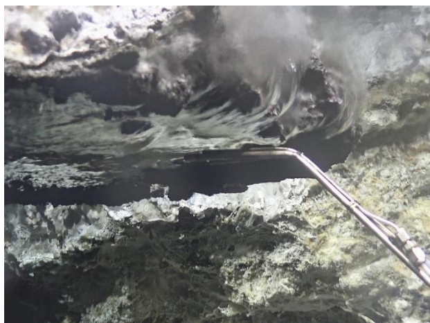
Figure 1: Sampling of a 289°C hot fluid at the Yggdrasil hydrothermal mound in 2900 m water depth with the intake port of the KIPS sampler. The hot fluid is reflected under a rock roof and flows directly upwards at the edge of the flange (© MARUM).
