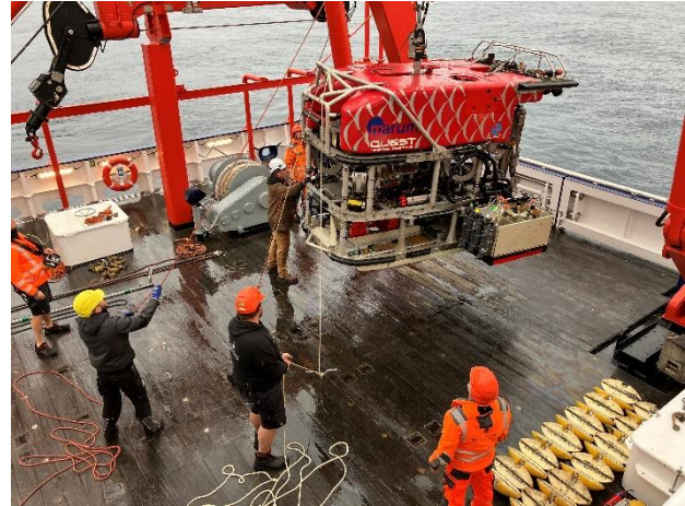
Figure 4: MARUM ROV QUEST is lifted up ready to enter the water and begin the first dive to the Jøtul hydrothermal field (© Gerhard Bohrmann).
