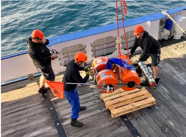
Figure 3: The AWI's first ocean bottom seismometer comes on deck, which was deployed in July 2023 during R/V POLARSTERN cruise PS137 in the area of the Jøtul hydrothermal field (© Gerhard Bohrmann).
