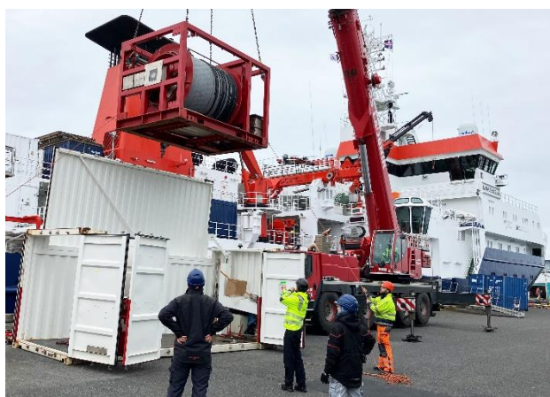
Figure 1: At the "Grandabryggja" pier in the Old Harbour of Reykjavik, a special crane hoists the 18-ton ROV winch onto the MARIA S. MERIAN (© Gerhard Bohrmann).
