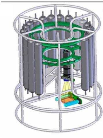
**Figure 6.** The UVP system in use on MSM130. View of the UVP lamps that illuminate a volume of seawater to allow camera to image particles and zooplankton (modified from Picheral et al., 2010, modified by Chris Galley).
