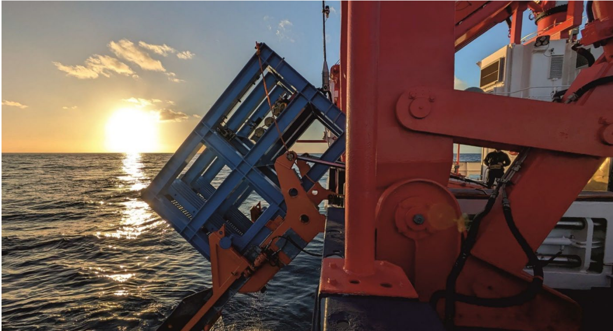
Fig. 1: In the last light of day, the test frame (here still without additional weight plates) on the hybrid cable comes back on board the research vessel MARIA S. MERIAN (Photo: M. Bergenthal)
