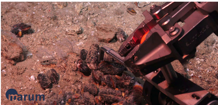
ISMS measurement of dissolved gases in seep fluids on top of Gigantidas mauritanicus bivalves at the Al Gacel mud volcano..
