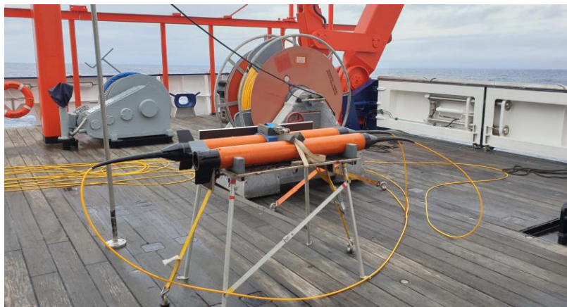
Magnetic gradiometer of the University of Hamburg; both sensors will be towed 300 m behind the vessel, being space at 100 m.
