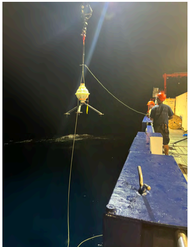
Deployment of an inverted echo sounder during the night (photo: Eleanor Frajka-Williams).
