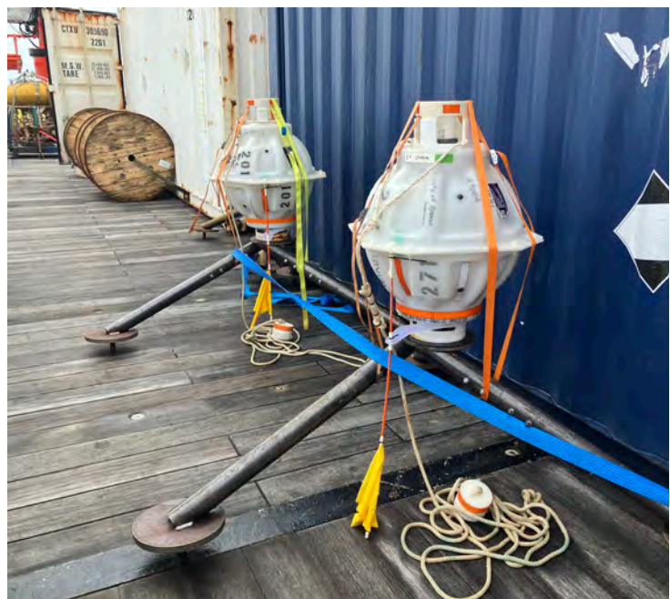
Inverted echo sounders with pressure sensors (PIES) on deck of Maria S. Merian, ready for being deployed. The devices are deployed with the hydrophone pointing upwards. For recovery the tripod is disconnected on an acoustic signal. On ascend the PIES turn around and the small flags point upwards for better retrieval (photo: Christian Mertens).
