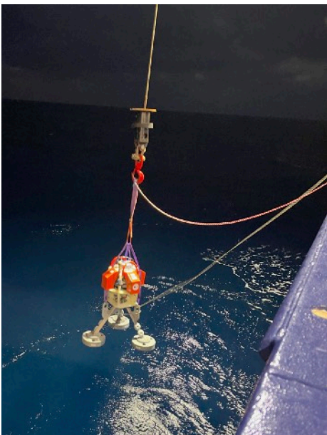
Lander (PIES) deployed close to mooring GB4. The instrument measures pressure at the seafloor and the travel time of acoustic signals from the seafloor to the surface and back (photo: Eleanor Frajka-Williams).
