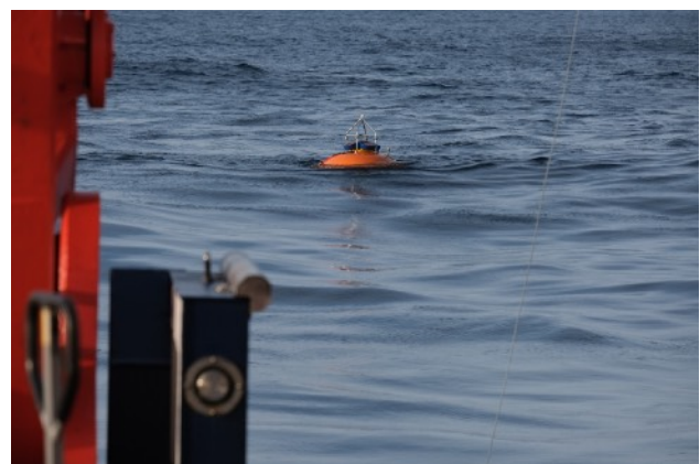
Top float with ADCP towed behind Maria S. Merian shortly after the start of the mooring deployment (photo: Christian Mertens).
