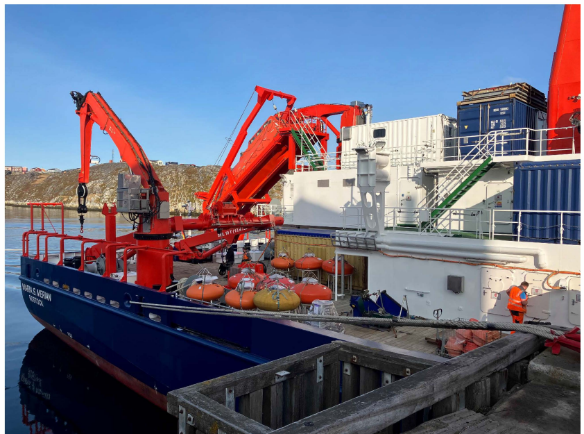
The research vessel Maria S. Merian in the port of Nuuk with the top floats for the moorings on the aft deck (photo: C. Mertens).
