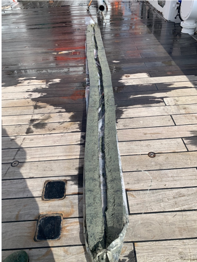
A 6 m long sediment core on deck of the Maria S. Merian, retrieved with gravity corer from the postglacial deposits covering the Late Pleistocene till layer. The sediments represent soft, bioturbated muds of middle (foreground) to youngest (background) Holocene age (Photo: R. Schneider).
