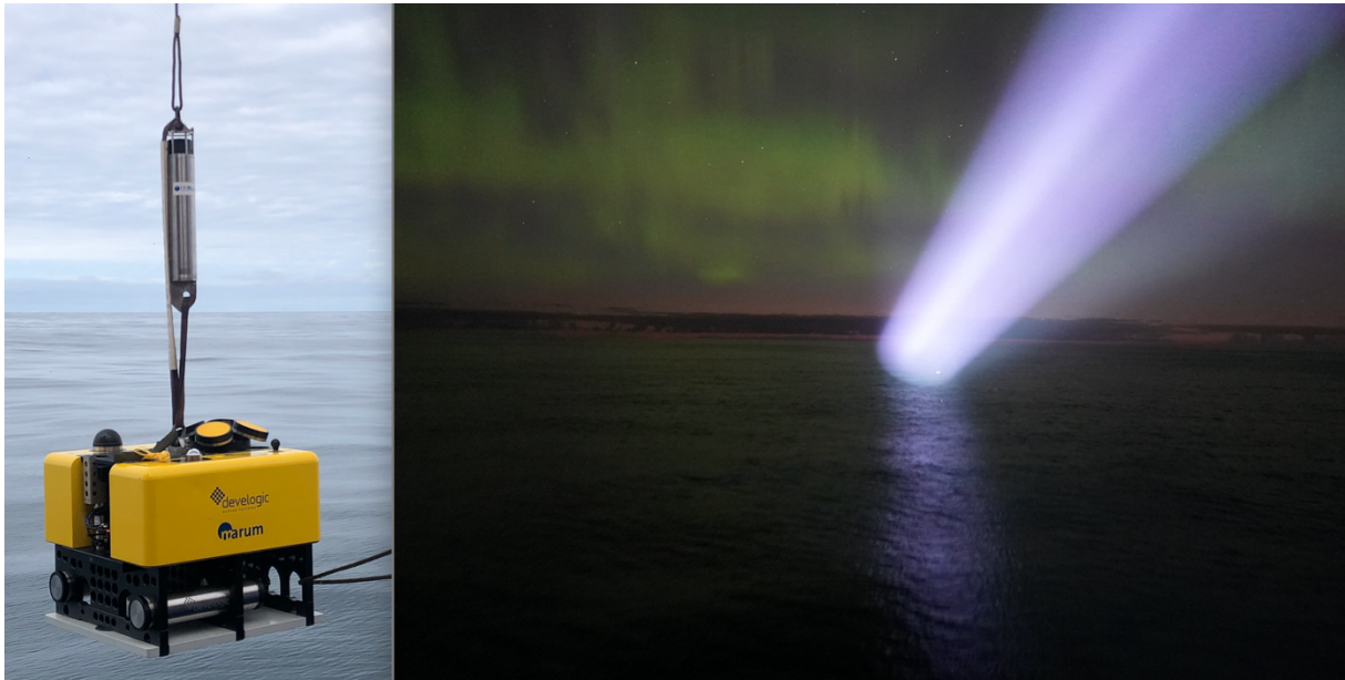
Figure 2 Left: MARUM Seafloor Lander during launch with the Releaser above it. Right: Under colourful Northern Lights skies, the lander surfaces and is followed by the beam of R/V MERIAN until it is safely recovered on board.
