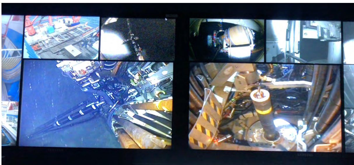
Figure 1 View of some of the control screens inside the MeBo control container. Here the pilots prepare the take-off maneuver back to the MERIAN. A borehole observatory can be seen on the bottom right with a white cover and yellow marking.
