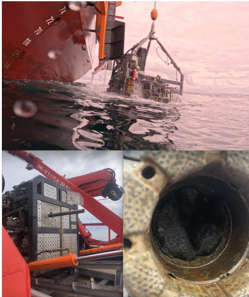
Abbildung 2 Above: MeBo recovery via the A-frame of the MERIAN. Bottom: The rig's terminal drill rod could not be stowed in the rig (left) because basalts blocked the core barrel (right).
