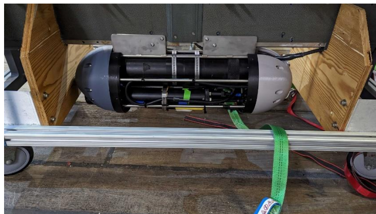
Figure 3: Sub mounted pCO 2 , TDGP, GPCTD/DO sensors.
