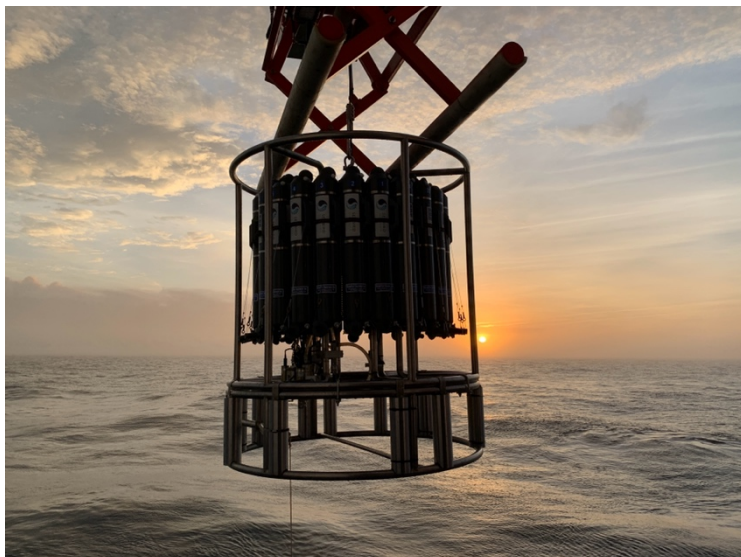
Fig.: CTD and Rosette water sampler deployed at a deep-sea station along the Halifax Monitoring Line (Photo L. deGelleke).
