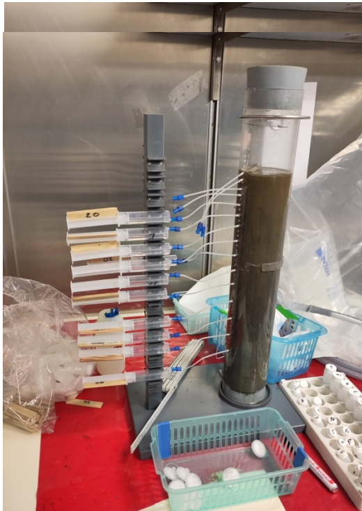
Fig. (left): Porewater extraction from a Multicorer with Rhizons in 1 cm intervals in the shipboard cool room (Photo F. Scholz)
