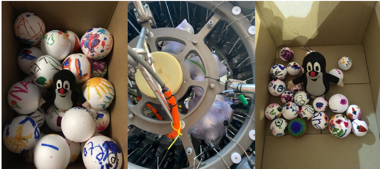
Fig. 3: The little mole with the styrofoam balls (before (after) they were tied to the CTD left (right)) shrunk at 5°S at 4200m depth under the high pressure of the water column. Picture: Joke Lübbecke
