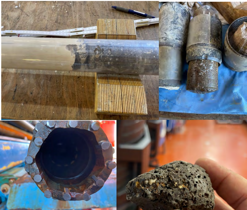
Fig. 1: Our inner cutting shoe after deployment in „Basalt“, Core with sediment overlying hard rock, weathered vesicular „basalt“ in core catcher and hand specimen. Photos: H. Pälke
