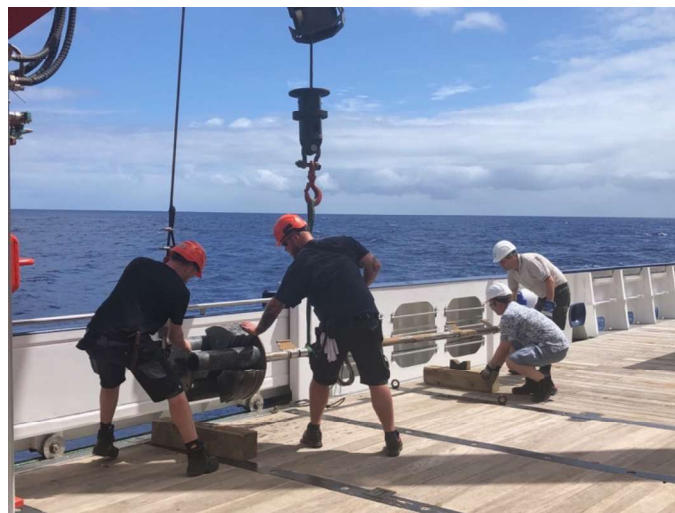
Figure 5: Recovery of the temperature loggers from the heat gradient lance. Photo: U. Röhl.
