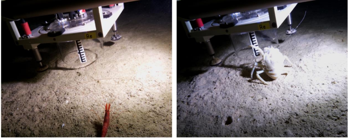
Fig. 2: Cylindrical flux chambers at the front of the Rover are inserted into the sediment to measure the total oxygen consumption of the enclosed sediment community. Some crustaceans escape these measurements and critically observe what happens.
