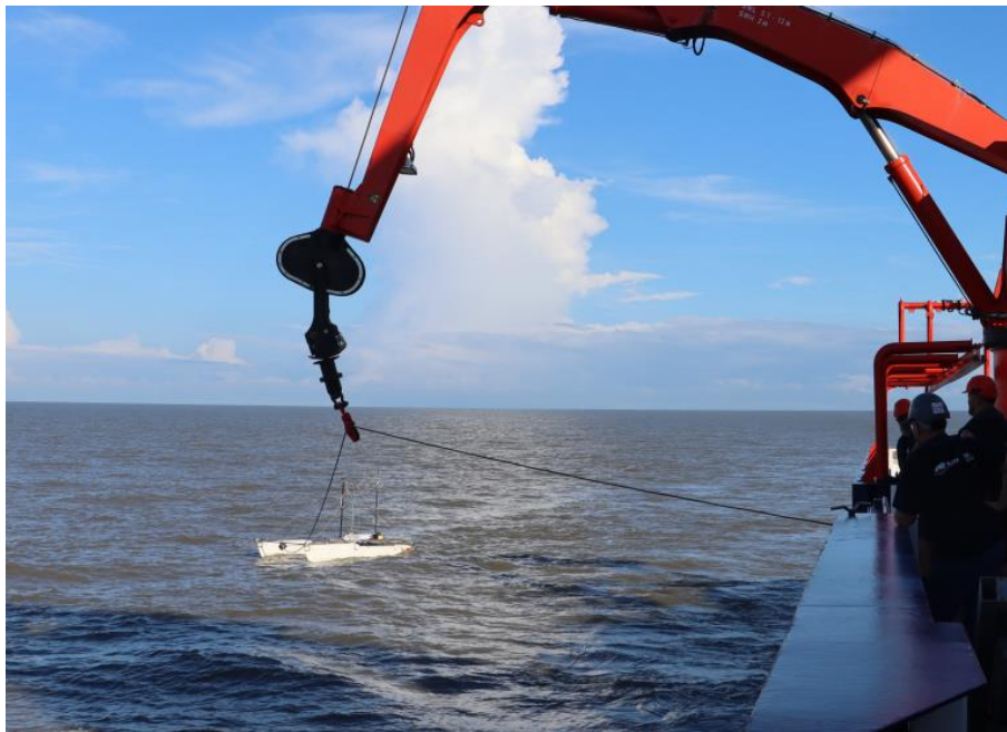
Figure 2: The towed catamaran with sensors for the measurement of near-surface currents and density stratification.
