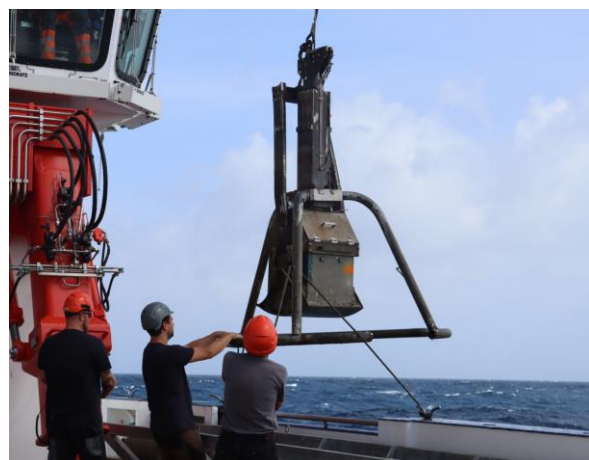
Left: "Winch stop", watching the rope tension diagram, the bottom contact of the instruments are monitored. Right: Well secured, a box grab arrives on deck. (Photos: C. Winter)
