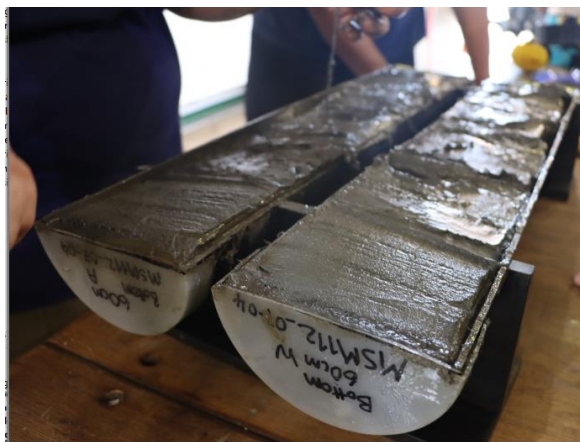
Left: A freshly split sediment core is prepared immediately after collection, Right: gravity sounder, box grab and the lander on deck of RV MARIA S. MERIAN during a quiet minute.
